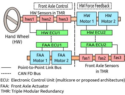
Fig. 3: SBW operational architecture.
