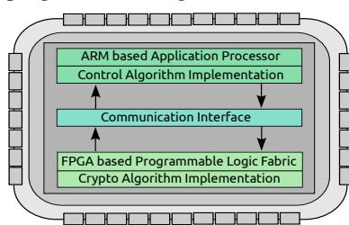
Fig. 1: High level architecture of proposed ECU.
