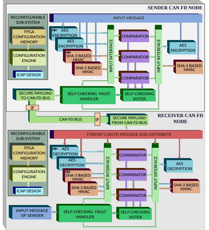
Fig. 2: Internal architecture of the secure and dependable cryptographic module (FT CM) implemented in PLF of the proposed ECU.
